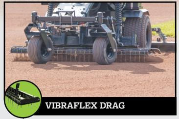
Our Vibraflex Infield Drag is a patent-pending attachment that re-imagines infield preparation. Evenly staggered U-pins transfer vibration and flex from front to back, dancing along the infield to shatter surface tension and prepare any engineered soil and surface conditioner. The Vibraflex Drag is endorsed by DuraEdge as the ideal attachment for preparing infield surfaces for the best possible safety and playability.
