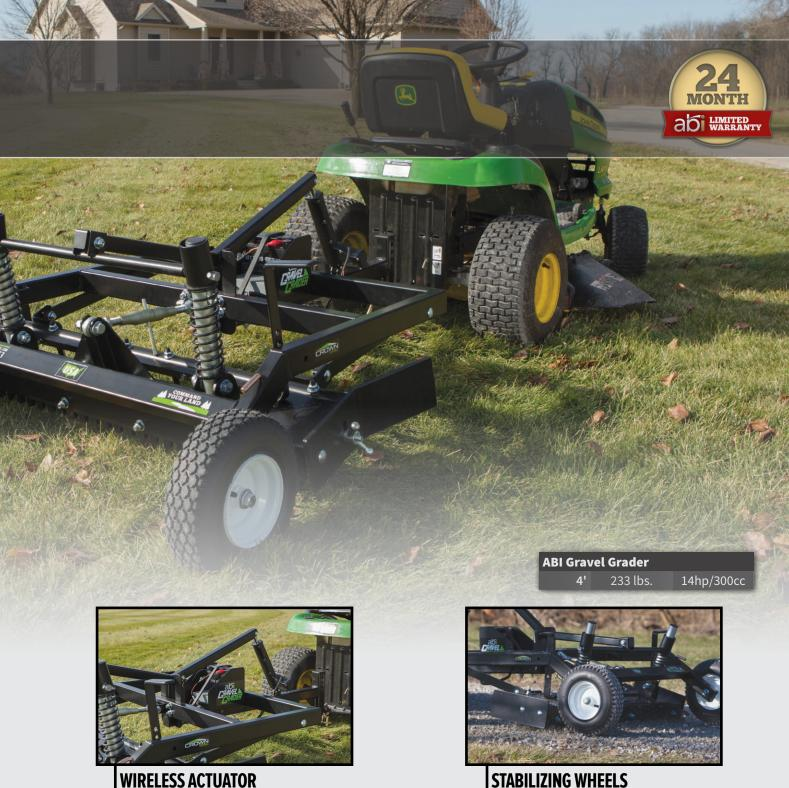
The wireless electric actuator easily dials in downward force on the springs and grading box. The hitch of the Gravel Grader tops out against the mower, using the weight of the operator and mower to put extra applied force into the loosening and grading action.
