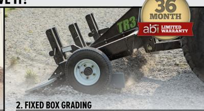
The TR3's leveling blade also locks into place for aggressive grading, similar to a box blade. Ideal for traditional "cut-&-fill" grading work. By carrying some material on the finish blade, users can also compact and level freshly loosened soil. The finish rake takes the TR3 above and beyond the typical box blade by providing a signature, even finish!
