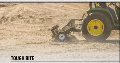
The TR3® Command Series attachment with hydraulic scarifiers penetrates 5 inches or more to remove compaction quickly. It reduces the labor and time needed for seeding jobs, all while creating perfect seedbeds for healthy, hardy growth!
