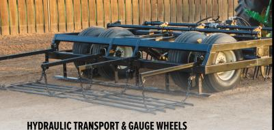
The hydraulic transport & gauge wheels are the "heart" of this Arena Drag. They support the weight of the Dragmaster and water tank during transport and use, and keep its loosening depth perfectly consistent with every pass.
