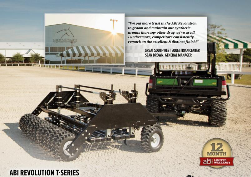
The ABI Revolution T-Series is the most effective pull-behind arena drag for high performance and synthetic footing arenas! Configurable in an 8 foot-wide model with a semi-mount hitch for tractors and caster wheels, or a 6-foot wide pull behind for large UTVs and small tractors with innovative walking-tandem axles. The ABI Revolution T-Series makes dialing in the perfect cushion and texture for your discipline a breeze!
