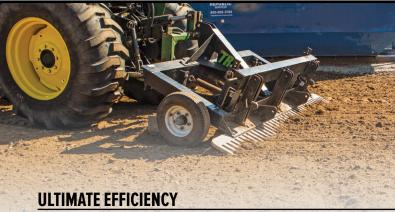
The TR3® was designed to sit at an angle so all ground contact points work simultaneously: loosen, level, and rake on every pass! Foam-filled stabilizing wheels work in tandem with the 3-point hitch to keep the tool level, making it easy to operate & achieve professional results!
