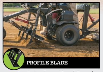
Occasionally de-compacting playing surfaces encourages proper moisture management and consistent ball play. ABI's patented Profile Blade attachment yields unparalleled de-compaction results by consistently slicing the profile of infield and warning track material from 1/2 to 3 inches under the surface. Profile Blades also cut weeds and grass at the root level, removing creeping grasses from infields and warning tracks.
