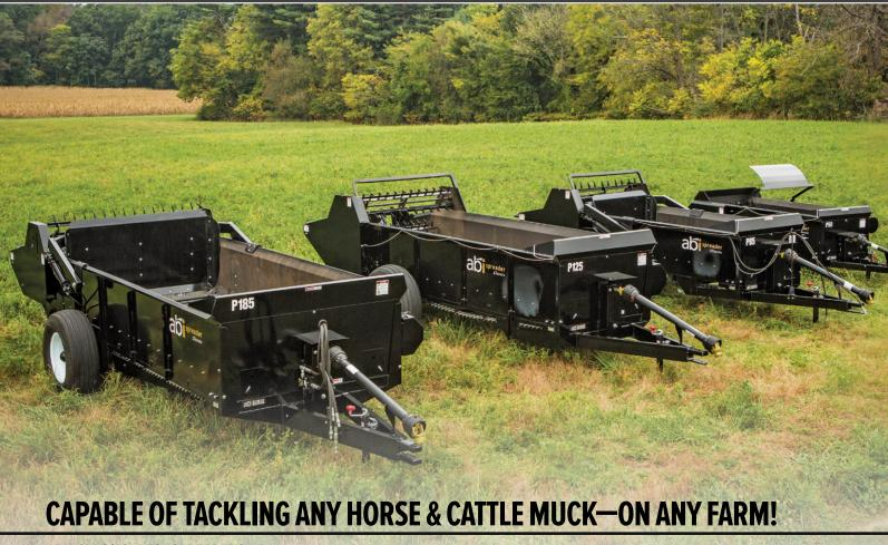
**ABI CLASSIC PTO SPREADERS** provide an even higher level of performance for tractors with a 540 RPM PTO (Power Take Off). The Classic PTO Spreader is ideal for extremely heavy loads where extra power may be needed or on terrain that is not conducive to good ground traction (such as extremely rough or hilly terrain, snow
