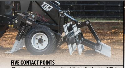
When equipped with the optional Profile Blades, the TR3 E - Trevor Brazile Edition has 5 points of contact with the ground! These independently adjustable components give you the control needed to groom, properly prepare, and renovate both the arena and the roping box, just like Trevor Brazile does in his personal arenas!
