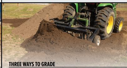
First, the TR3's leveling blade can float to automatically catch high areas and gently drop material into lower areas. Secondly, the TR3's leveling blade also locks into place for aggressive "cut-and-fill" grading, similar to a box blade. Finally, pushed backwards, the TR3 cuts high spots, piles debris, or fills in landscape edges when pushed backwards, all while the stabilizing wheels prevent gouging!
