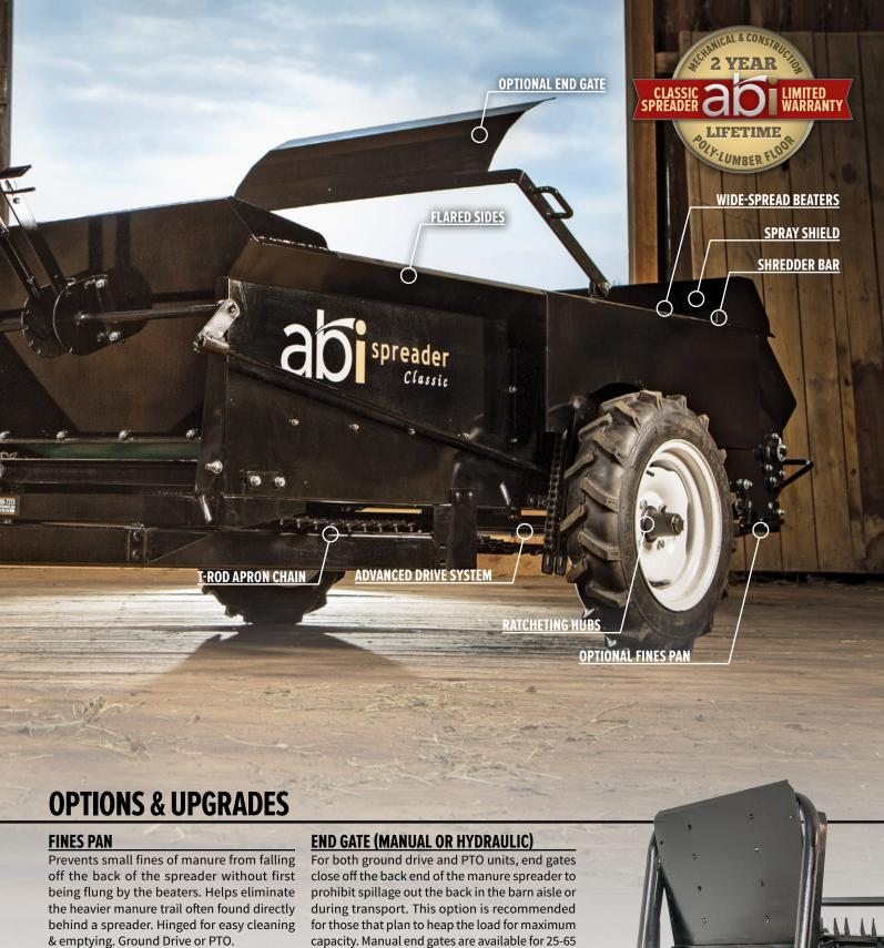
ft<sup>3</sup> units. Hydraulic end gates are available for 25-65 ft<sup>3</sup> units. Hydraulic end gates require one set of hydraulic ports on a tractor, and are available for 85, 125, & 185 ft<sup>3</sup> models (2 total sets of ports required for 185 ft<sup>3</sup> model). Hydraulic end gate shown.
