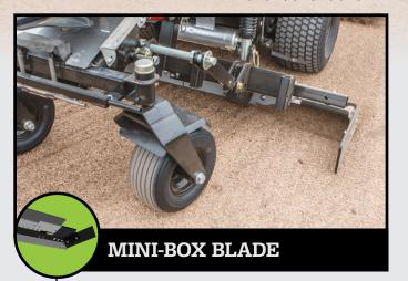
ABI's Mini-Box Blade attachment gives the Force extra earth-moving muscle and unmatched versatility. With fingertip control and perfect visibility of the powerful hydraulic and springloaded arms, users can quickly and effectively carry material, grade, and level with finesse! For ultimate control, pair the Mini-Box Blade with ABI's laser system (see page 74).
