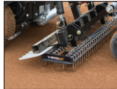
VIBRAFLEX 5800 60" Wide | 1/2" Spacing | 1/8" OR 1/4" Pins
