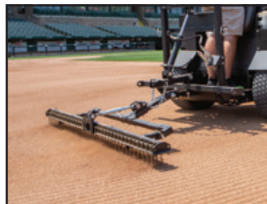
VIBRAFLEX 3500-R 72" Wide | 1/2" Spacing | 1/8" or 1/4" Pins
