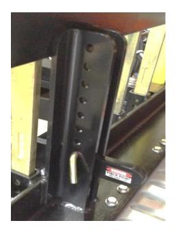
Step 2 – Remove the ½" bent pins from the upright mast on the back that is locking down the leveling blade. If these pins are already at the top of the mast up then skip this step and move on to step 4. If the pins are in place and cannot be removed from the uprights, then the TR3 may need to be lowered to the ground to take the pressure off the pins. Remove the pins and pin each one in the top hole on the uprights. Make sure to secure the bent pin back using the provided lynch pin.
