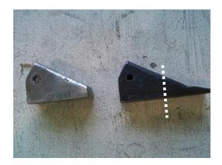
The tip on the left is worn and the right is new. The white line shows the maximum wear point before there is damage to the shank. Going much higher than the white line will mean that the shank will need to be replaced.
