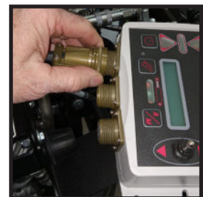
Fig 23. Tab on ports to line up with slots on cable plugs
