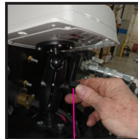
Fig 19. Thumb screw on pivoting extension post
