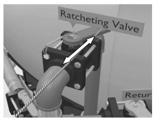
To ensure the sprayer is "on" make sure the silver "eared" tab is fully in line with the tubing.
