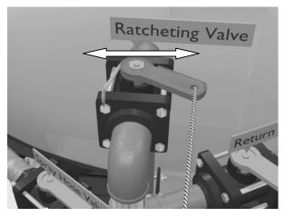
To ensure that the sprayers are "off" make sure the silver tab is not in line with the tubing. The tab will run perpendicular to the tubing.
