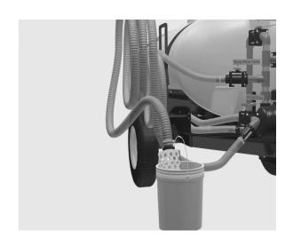
Before using the Pond Fill option, secure the end of the attachment in a 5-gallon bucket. This is to help prevent debris from entering the system and damaging the poly pump.
