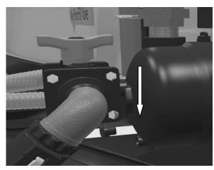
Remove this plug from the Poly pump to drain out water from the Poly pump before storage, changing water sources, or cleaning. Replace the plug back into the poly pump before using the Water Trailer.
