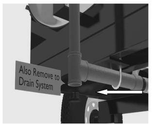
To drain water from the piping and spray boom line, remove this plug and allow any excess water to drain out. Replace plug before using the Water Trailer.
