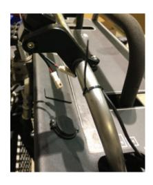
5. Place magnet on edge of hub as shown. Do not line up directly over sensor or sensor will count double.
