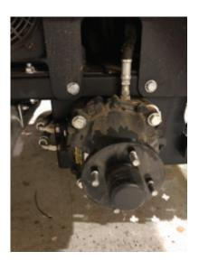
2. Remove top rear transmission mount bolt and install sensor bracket in place of washer on bolt. Position sensor from speedometer kit near wheel hub as shown.
