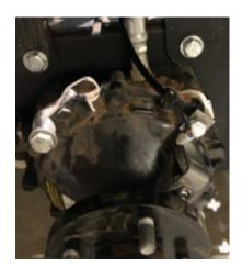
3. Install handle bar mount and back plate to Speedometer as shown. Use provided foam spacer to install to LH side of speed lock bar, then trim spacer as needed.
