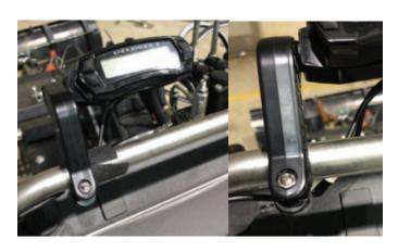
4. Route sensor cable through opening in fender and along side engine air filter to exit beside dash. Ensure cable can't be pinched and use provided zip ties to secure and plug into speedometer.
