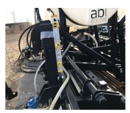
Step Three: After attaching your tractor to the three-point of the Speedmaster use your top link and adjust it so that the three-point mast on the tool is running level vertically. If you have it angled backward too far you can possibly put extra strain on the rolling basket and can cause damage. This also sets the rest of the ground engaging components to work together properly.
