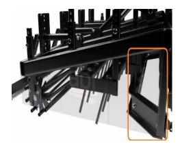
Step Seven: The Speedmaster leveling blade (circled in orange in the picture) is controlled hydraulically from the seat of the tractor by the operator. The operator can lower the blade at the high spots and raise the blade to fill in the low areas in the arena footing.
