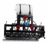
Step One: Connect the three-point of your tractor to the Speedmaster. The red circles in the pictures are highlighting where the connections are located on the unit.
