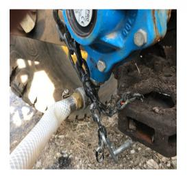
Step Two: Attach the PTO pump by pulling back on the locking collar, align the splines of the tractor with the splines on the pump and slide it on as far as it will go. Next, slide it back until you hear the lock latch click in place locking the pump to the tractor PTO shaft. Last be sure to securely chain the pump to the tractor to prevent it from spinning. Be sure to idle the tractor down low before engaging the PTO and then idle up to desired speed. Maximum of 540 RPM.
