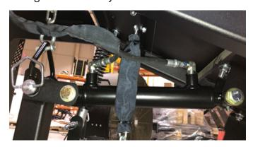
5. The single link mounts the same way on the left side of the machine at the highest point.
