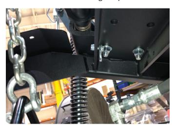
6. Connect Snap Link to Single Chain Link for storage, being sure not to capture any hoses.
