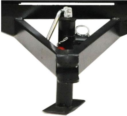
The swing away jack is used to hold the spreader in a safe level position when not connected to a tow vehicle. Use the jack to raise or lower the spreader for easy connection to the tow vehicle. To rotate the jack remove the attached pin from the holder, rotate, and reinsert pin. To keep the jack from catching during use, always raise and rotate the jack before operating the Spreader.
