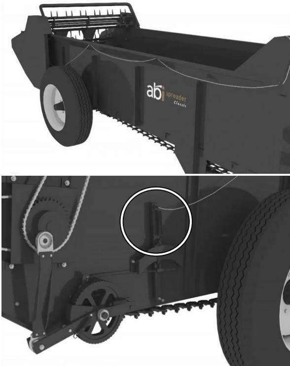
The speed adjustable rope controls the speed of the apron chain. Pull the rope forward slowly to allow the lever to lock into each slot as you pull forward. This allows for multiple spreading speeds. When you want to stop the apron chain pull the rope fully forward and allow the lever to fully reset. This will disengage the apron chain.
