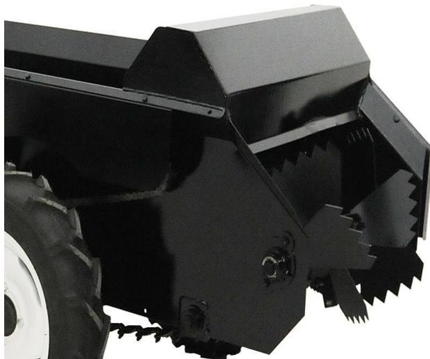
This exclusive feature offers two features. First is to prevent any manure from flowing over the beaters and shredder bars, and second it acts as a shield for spray off. This helps with “clean” spreading, and prevents spray off from hitting the operator.
