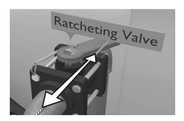
To ensure the sprayer is "on" make sure the silver "eared" tab is fully in line with the tubing.
