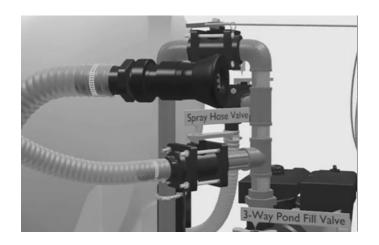
Adjust the pressure coming from the nozzle by twisting the nozzle open or close. Remember to hold on tightly to the hose when using the Spray hose for safety purposes. When connecting the Spray nozzle hose to the male quick connect fitting, ensure the rubber seal is firm seated in the female quick connector. If the seal is not firmly seated, the hose may lose pressure.
