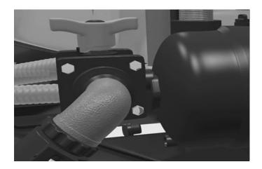
Remove this plug from the Poly pump to drain out water from the Poly pump before storage, changing water sources, or cleaning. Replace the plug back into the poly pump before using the Water Trailer.
