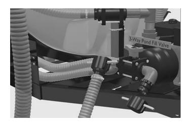
Before using the Pond Fill option, secure the end of the attachment in a 5-gallon bucket. This is to help prevent debris from entering the system and damaging the poly pump.
