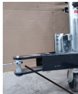
Rotate top nut counter-clockwise to wedge top and bottom hitch bars apart until hitch can slide between bars. Remove bolts, washers and nuts and position hitch as mentioned above.
