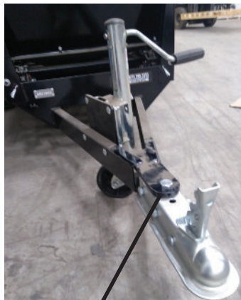
Bolt goes thru back hole in hitch.
