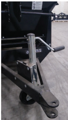
Bolt goes thru back hole in hitch.
