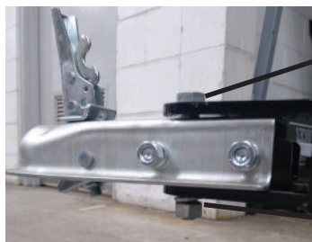
Bolt goes thru back hole in hitch.
