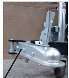
Rotate top nut counter-clockwise to wedge top and bottom hitch bars apart until hitch can slide between bars. Remove bolts, washers and nuts and position hitch as mentioned above.
