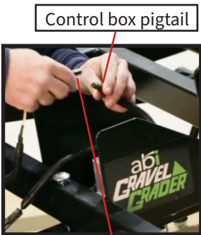
Fig 3. Control box pigtail 8' wire harness
