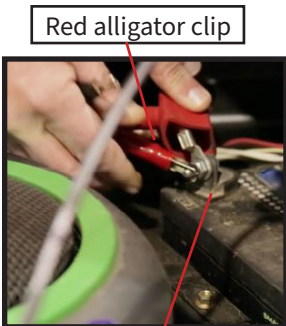
Fig 5A. Red alligator clip Tow vehicle positive battery terminal
